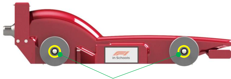
View of wheels only obstructed by wheel support system (circled in yellow)
